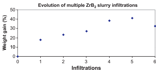
Fig. 5. Evolution (wt.% gain after drying based on a untreated tube) of multiple infiltrations by ethanol-based ZrB 2 -slurry.
